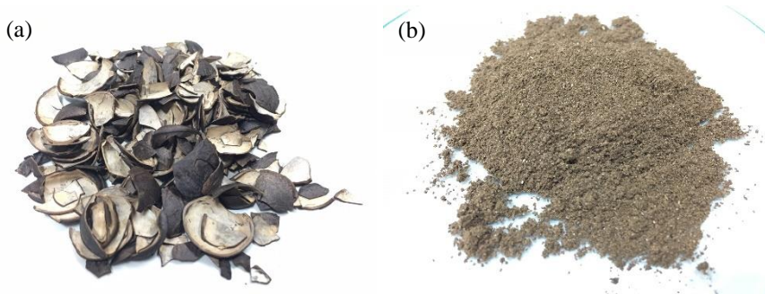
Fig. 1. Sacha inchi shell (a) soaked and dried biomass (b) grounded biomass size 106-425 \mu\text{m}
